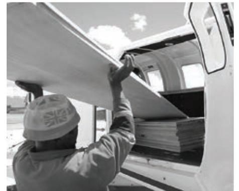
ramp enabling the XSTOL™ to be quickly loaded and unloaded. The configuration of the aircraft can be quickly changed between passenger and cargo roles within 30 minutes. All the standard passenger seats can be removed and stowed in either the storage compartment at the rear of the cabin, or in the cargo pod for quick conversion between roles on return legs.
