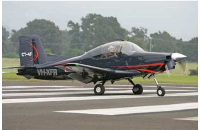
All of the Akala's electronics (left) and the big Lycoming, coupled with the wing being eight centimetres further forward than earlier CT-4 variants, makes for heavier nose wheel steering (right).
