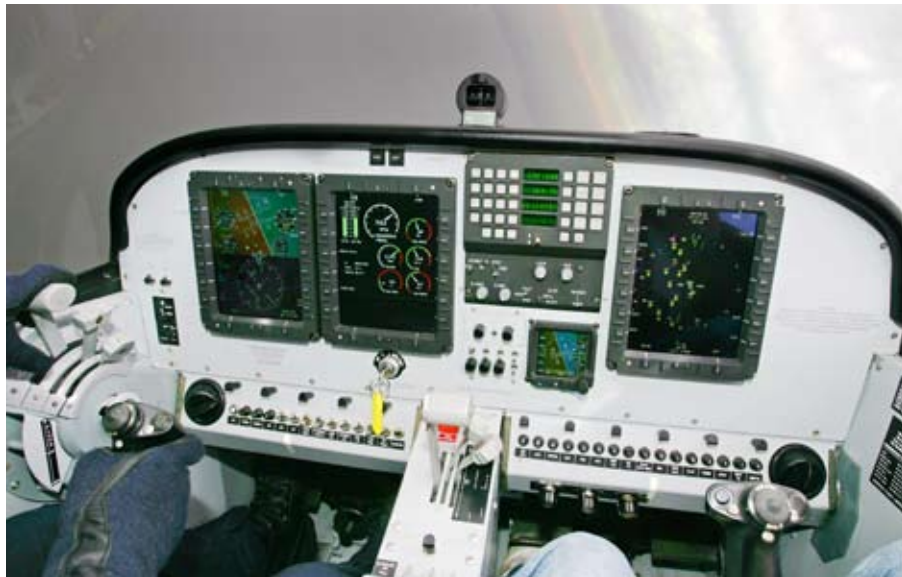
(left) The CT-4F's cockpit resembles that of the T-6B Texan II (right) with its three multifunction display screens, a five-in-one backup flight instrument, and the up front control panel making the transition for a student between the two types very easy.
