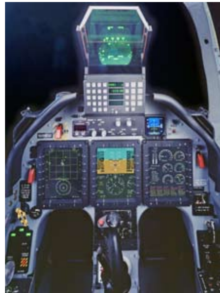
(left) The CT-4F's cockpit resembles that of the T-6B Texan II (right) with its three multifunction display screens, a five-in-one backup flight instrument, and the up front control panel making the transition for a student between the two types very easy.
