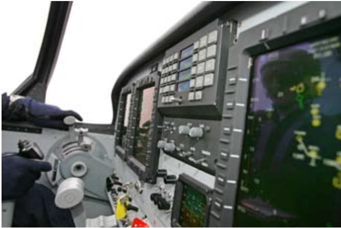
All of the Akala's electronics (left) and the big Lycoming, coupled with the wing being eight centimetres further forward than earlier CT-4 variants, makes for heavier nose wheel steering (right).
